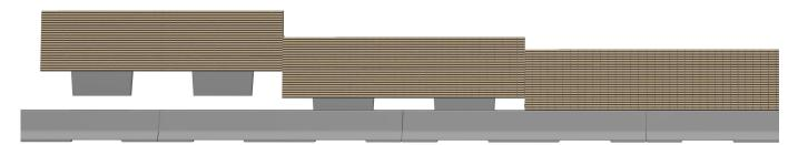
The REBLOC® Integrated Noise Barrier consists of a base element of New Jersey profile and a plate-shaped noise barrier element. The slim total system width makes optimum use of the space available. One noise barrier element is inserted overlapping
